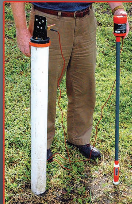
Potential meter with optional 30" electrode extension
